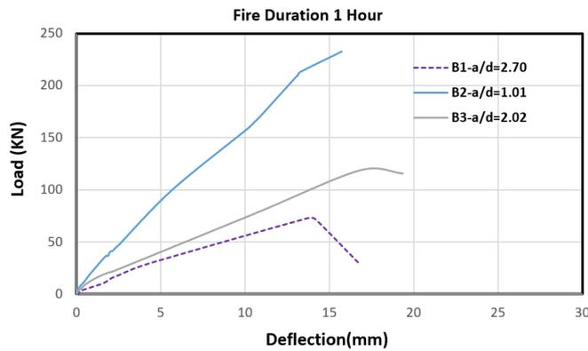
Fig. 9: Load-Deflection Curves at Mid Span for Beams Tested.
