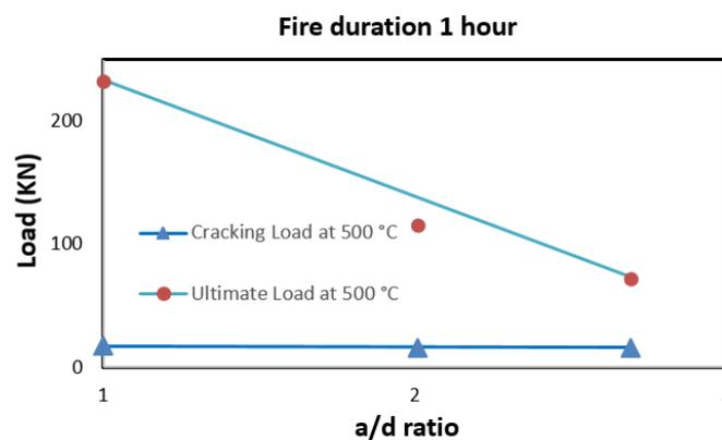
**Fig. 7. Effect a/d ratio on Cracking and Failure load.**
