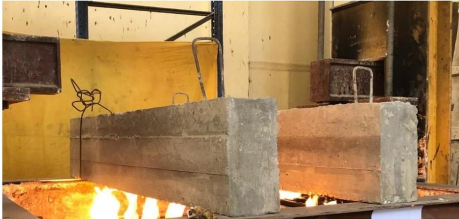
Fig. 5. Beams subjected to Fire.
