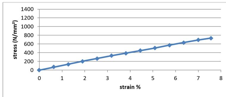
**Fig. 2. Stress-Strain Curve for Glass Bar**
