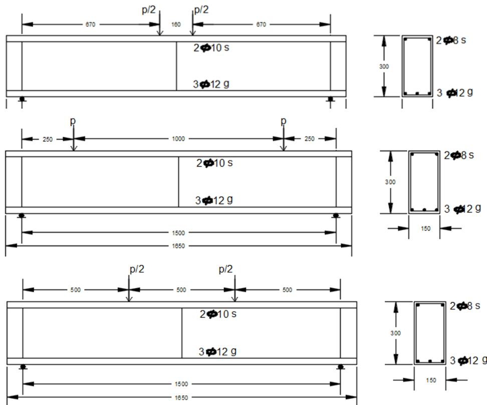
Fig. 3. Details of Tested Beams.
