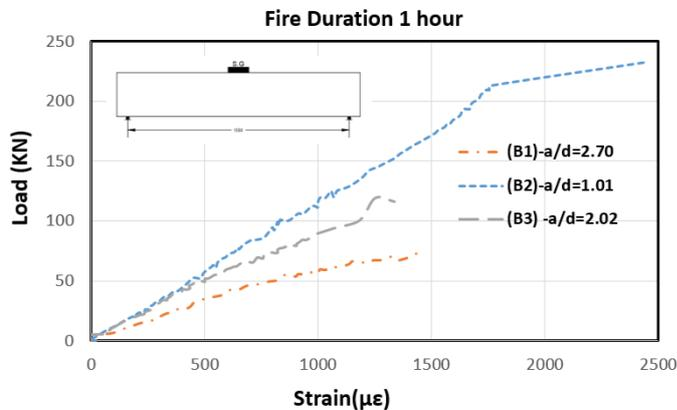
Fig. 10. Load-strain relationship for the concrete at top compression zone.
