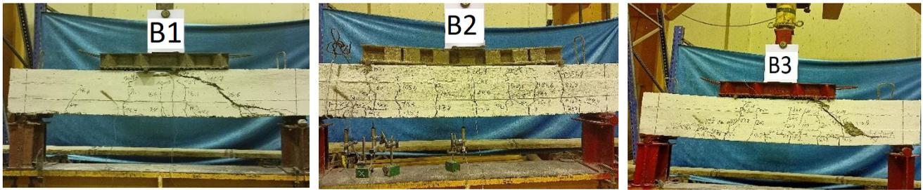
Fig. 8. Crack pattern and Failure Mode of Tested Beams.
